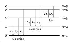
emitted due to the jump of electron from the *L*, *M*, *N* shells to the K-shells gives  $K_{\alpha}$ ,  $K_{\beta}$ ,  $K_{\gamma}$  lines of the *K*-series of the spectrum.
