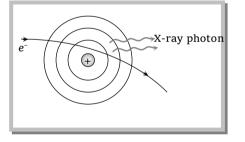
*Note* : Continuos X-rays are produced due to the phenomenon called "Bremsstrahlung". It means slowing down or braking radiation.
