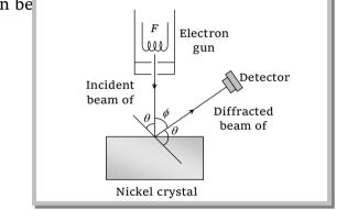
The diffracted beam of electrons is received by the detector which can be positioned at any angle by rotating it about the point of incidence. The energy of the incident beam of electrons can also be varied by changing the applied voltage to the electron gun.
