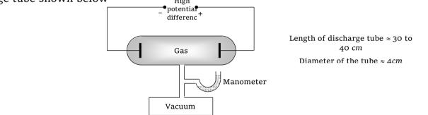
The discharge tube is filled with the gas through which discharge is to be studied. The pressure of the enclosed gas can be reduced with the help of a vacuum pump and it's value is read by manometer.
